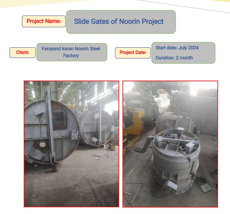
Execution of cutting, installation, welding and grinding operations, including argon porous plugs and base plates, slide gates mechanism of melt shop ladles 7 sets. Design and engineering by Sarralle company from Spain.
